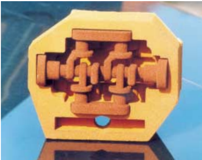
Mould and core for hydraulic casting made by SLS
